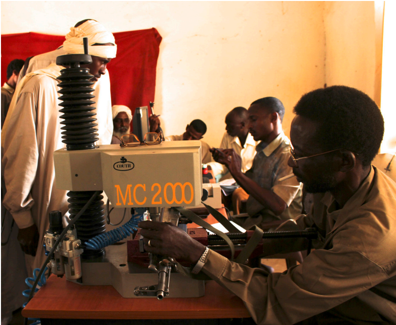
Couth MC2000 dot-peen percussion marking machine in use. (C) Nikhil Acharya/ BICC
